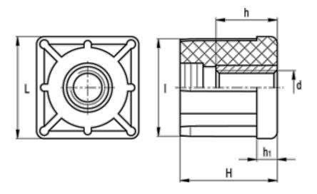
$\begin{array}{lll} d & = M10 \\ h & = 10 \\ H & = 38 \\ h1 & = 8 \\ Internal tube size = 37.6 \\ I & = 37.6 \\ L & = 40 \\ \end{array}$
